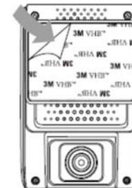
Peel of the protective paper from the mount to reveal the adhesive surface.
