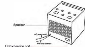
Speaker, USB charging port, AC power cord, FM wire antenna
