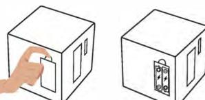
Step 1 Take off the cover on the bottom of unit. Step 2 Insert new battery into battery compartment with the correct pole.
