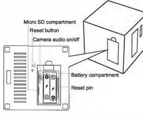
Micro SD compartment, Reset button, Camera audio on/off, Battery compartment, Reset pin
