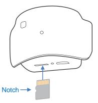
To remove the card, simply push it further in again so it toggles back out.
