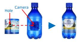
Since the function S button will be hidden behind the label, you will have to poke around about half inch above the camera hole until you feel it click. It should be right on top of the "tto" at the end of the word "SanBeweketto".
