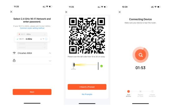
(5) After hearing the prompt, the device indicator changed into green from red, finish the network connection then click done as the following picture.
