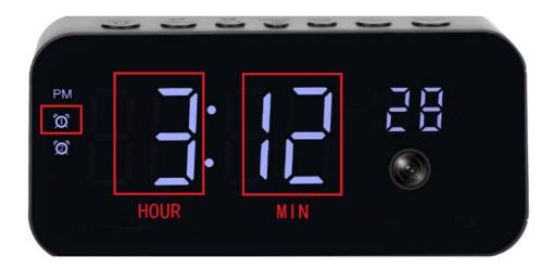
Press the "MIN" to increase the clock by minute. Press and hold - time to increase rapidly.
