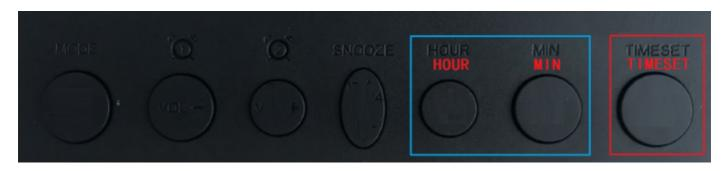
1. TIMESET: Press and hold the "TIMESET" for 3 seconds to enter the time setting.
